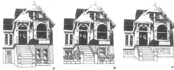
4.4 Different types of built bases: a. full-story base; b. half-story base; c. crawl space.
